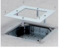
Preparation of an underfloor system Mounting the heavy-duty blanking lid on the underfloor box. Adjust the support feet to the right height and secure with a locknut.
