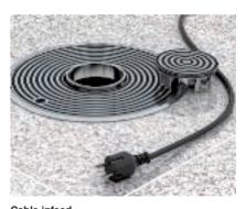
The consumer cables are inserted through the opened tube body with the opened lid and then connected in the installed connection sockets. Then the lid is pushed down and locked and the tube body cover attached.
