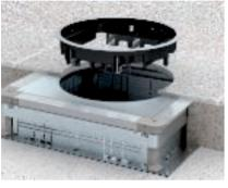
**Mounting in duct systems** Insert the service outlet into the mounting lid from above and screw it tight. The fastening unit grips under the mounting lid.
