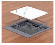
Adjust of the floor covering recess to 8 mm for GES4-2, GES6-2 and GES9-2 Slacken the 4 lid screws and the inserted 5 mm spacer frame and replace it with the 2 mm spacer bars. Screw the sheet steel lid on again.
