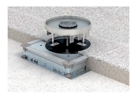
Height-adjustable round heavy-duty cassettes are suitable for flushfloor device installation in raised and cavity floors and in all kinds of screed-flush installation systems in dry or wet-cleaned floors with high traffic loads. The cassettes are designed for individual static loads of up to 20 kN (load class 2). The interior height adjustment allows exact adjustment of the top edge of
