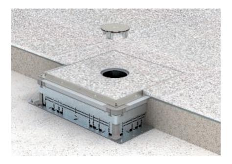
Heavy-duty frame cassettes are suitable for the top closure of an underfloor draw and junction box in dry or wet-cleaned floors with high traffic loads. The cassettes are designed for individual static loads of up to 10 kN (load class 1) or 20 kN (load class 2). Additional heavy-duty supports in the box body ensure the necessary stiffness and load capacity. The cassettes are fastened directly on
