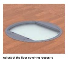
10 mm Slacken the 4 lid screws and the inserted 7 mm spacer frame and replace it with the 2 mm spacer bars. Screw the sheet steel lid on again.
