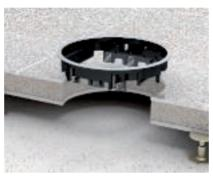
Mounting in raised and cavity floor. When used in raised and cavity floors, the universal fixing bracket acts as an expansion claw. Tighten the screw with max. 4 rotations. The claws fasten the service outlet in the mounting opening.
