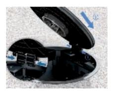
**Installation of the hinged cover**Push the hinge together and insert in the holder in the frame.
