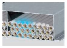
The space requirements of the cables in the UFS ducts with empty spaces
