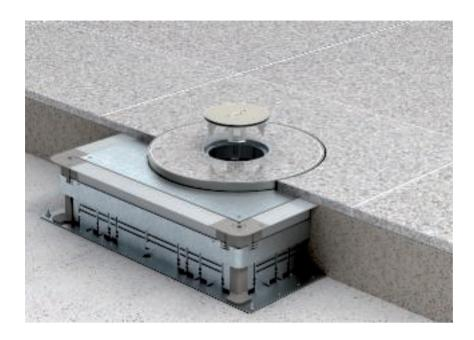
Height-adjustable round cassettes are suitable for flushfloor device installation in raised and cavity floors and in all kinds of screed-flush installation systems. Depending on the design, they are suitable for dry, moist or wet-cleaned floors. The interior height adjustment allows exact adjustment of
