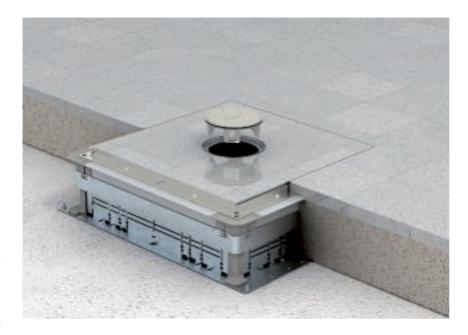
Frame cassettes are suitable for the top closure of an underfloor draw and junction box in dry, moist or wet-cleaned floors. They are fastened directly on an underfloor junction and branch box without the use of a blanking lid. The cassette frame is fastened to the box body using four fastening screws
