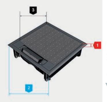
Various installation and floor cut-out dimensions must be taken into account for the mounting of service outlets and the application of floor coverings in the device lids.
