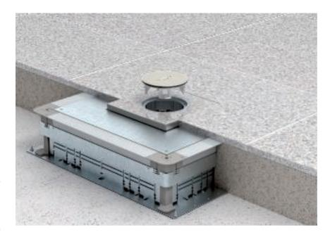
Height-adjustable square cassettes are suitable for flushfloor device installation in raised and cavity floors and in all kinds of screed-flush installation systems. Depending on the design, they are suitable for dry, moist or wet-cleaned floors. The interior height adjustment allows exact adjustment of
