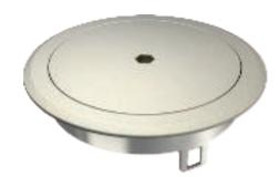
Blanking cover with Allen slot for GES R2 floor socket for direct installation in the MT R2 installation socket. The lid exit can be used as a cable outlet. When closed, the floor socket fulfils the requirement of EN 50085-2-2 for wet-cleaned floors.
