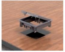
**GES mounting in raised floor**When used in raised floors, the fastening bracket reaches under the raised floor plate, fastening the service outlet.
