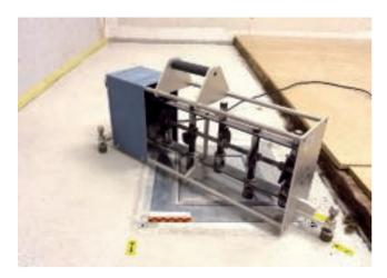
The underfloor systems from Ackermann made by OBO are, amongst other things, intended for installation in floating wet screeds. Normally, there are requirements for the transmission of air and footfall sound, both for vertical sound transmission, i.e. from storey to storey, and for horizontal sound transmission, i.e. from adjacent rooms.
