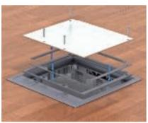
Adjust of the floor covering recess to 3 mm for GES4-2, GES6-2 and GES9-2 Slacken the 4 lid screws and the inserted 5 mm spacer discs and replace them with the 2 mm spacer discs. Screw the sheet steel lid on again.
